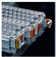
To ensure high energy density and safe battery operation, clean contact points are a must for the electrical connection between the battery cells and the arrester, in this case a lead frame.
