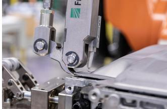
A tool dubbed "Knacker" was developed to prize apart the adhesive bonds between the upper and lower shell of a battery. Source: Fraunhofer IPA/Photo: Rainer Bez
