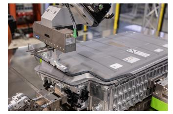
The project developed a variety of hardware for automated disassembly tasks, such as this small parts gripper. Source: Fraunhofer IPA/Photo: Rainer Bez
