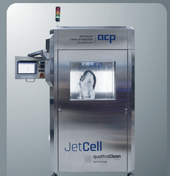
JetCell - Flexible automated cleaning cell, inline or stand-alone with application specific configuration
