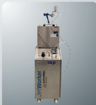
JetWorker - Mobile snow-jet cleaning system, with static nozzle or hand-held system
